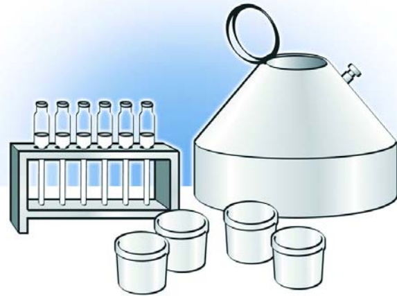
Butyrometer is used to measure fat content of milk
