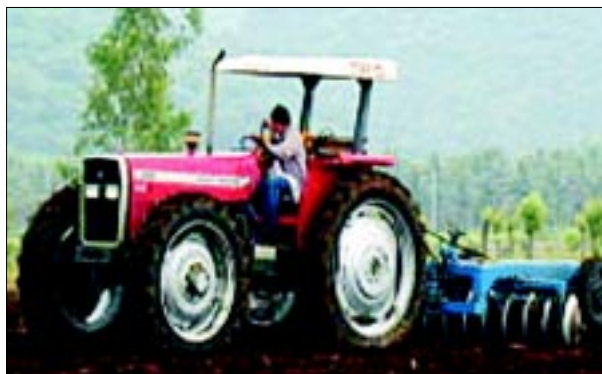
Fig. 9. Disc harrows being used to loosen hard layers exposed due to shifting of soil.
