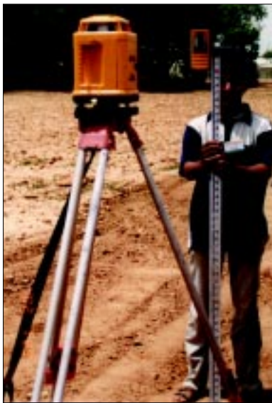
Fig.16. Checking the laser transmitter and receiver communication for actual field survey.
