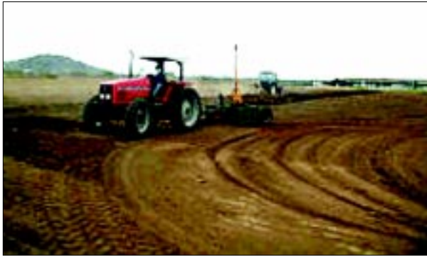
Fig.19. Tractor should be driven in circular direction in the field from high to lower areas.
