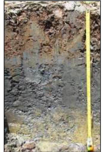
Fig 1. Soil profile with a blue-gray colored layer indicting poor drainage
