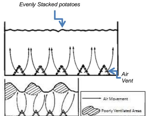
**Figure 14.** Distribution of potatoes in a storeroom affects ventilation. Triangles in the drawing are basal air ducts. The figure at the top shows evenly distributed potatoes receiving equal air circulation throughout the pile. The bottom 2 figures show uneven piles and area of the pile that will receive poor air flow. (Source: CIP. 1981. *Principles of Potato Storage*. Lima, Peru: International Potato Center (CIP) 105 pp).
