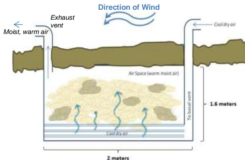
Figure 5. Example of underground storage with ventilation. Source: CRS
