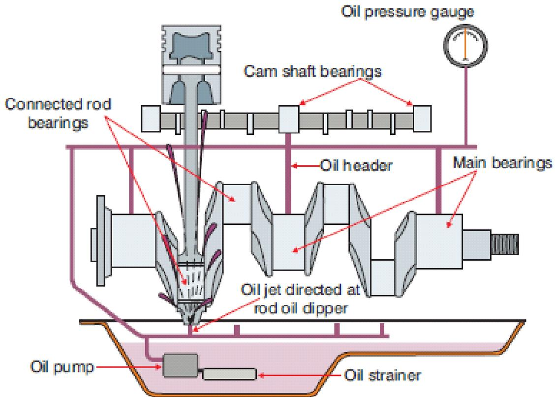
**Oil helps to seal rings, clean and cool parts, and reduce friction.**
