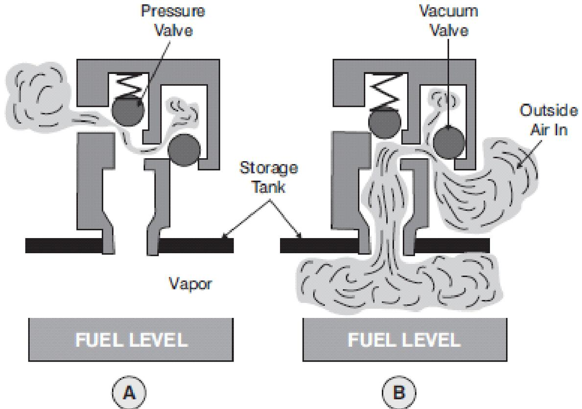
When tank pressure rises above 3 psi (21 kPa), ball on pressure valve rises and allows enough gasoline vapor to escape to keep pressure at 3 Psi.
