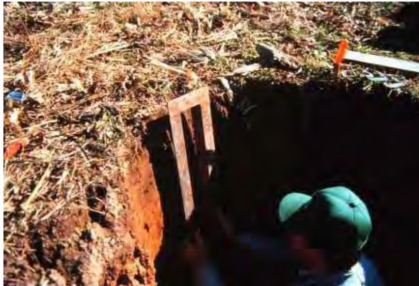
**3.) Insert the cutting edge into the profile-face to mark the edges of the frame (hammer or other pressure).**
