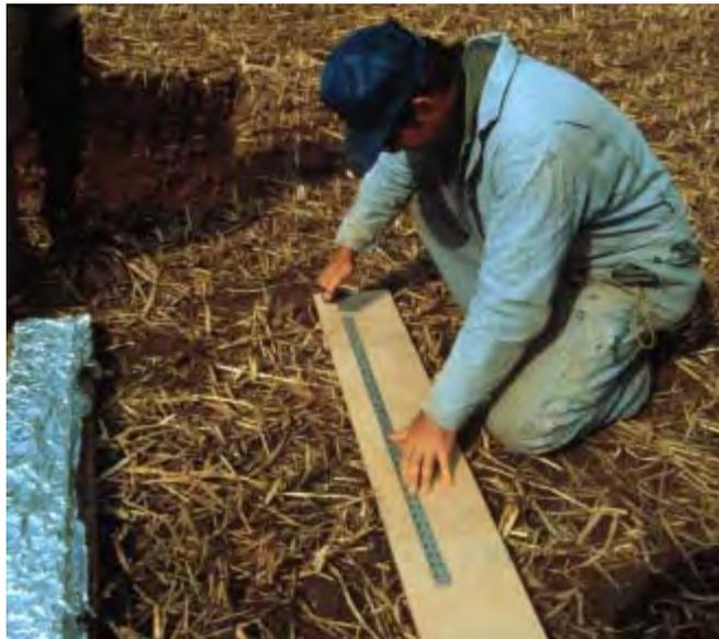
**12.) Prepare mounting board (cabinet grade plywood 3/4"x 8" x 48" is used) by outlining, in pencil, the 4' x 40" area to contain the monolith on both sides of the board.**
