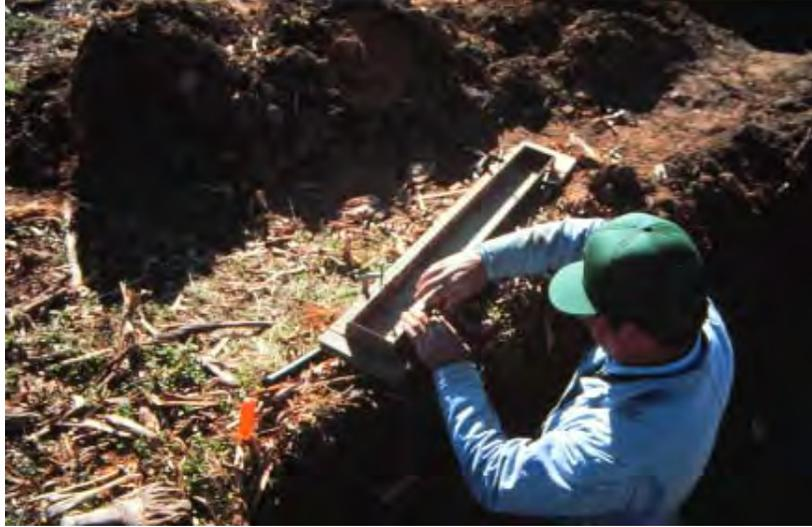
**6.) Attach a flat board (approximately 3/4" x 8" x 48") over the flat side of welded angle iron frame with C-clamps.**
