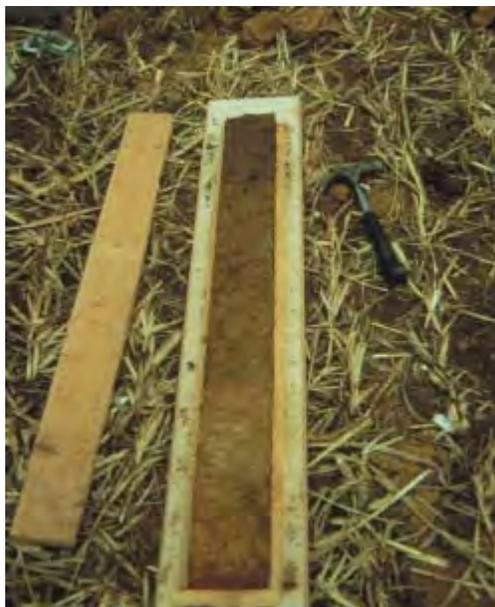
23.) Allow soil monolith to air dry for 2-3 weeks - it is absolutely essential that all moisture be removed from the monolith before applying "hardening compound", otherwise very undesirable and almost irreversible chemical reactions occur.
