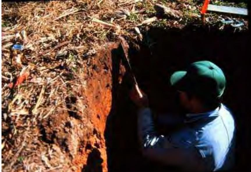
**4.) Remove frame and carve the profile to be captured from the pit face by removing soil from the area to the outside of the marked profile.**
