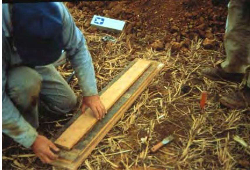
**19.) Place a piece of board (cut to pass through the metal frame) on the soil profile exposed inside the frame.**
