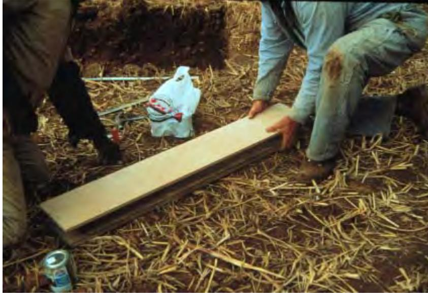
**16.) Align mounting board with soil profile and depress board with protruding nails into the profile with firm even pressure. Take steps to insure board is squarely aligned with profile before applying firm pressure.**
