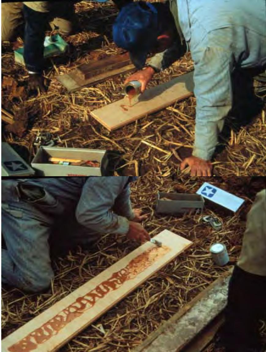
**15.) Also apply a generous coat of Elmer's Contact Cement to the smoothed soil profile face exposed in the frame. (Usually, this must be accomplished in less than 15 minutes due to rapid drying time- some folks also choose to place 1-2 layers of cheesecloth between the board and the profile as an interface to hold additional glue.)**
