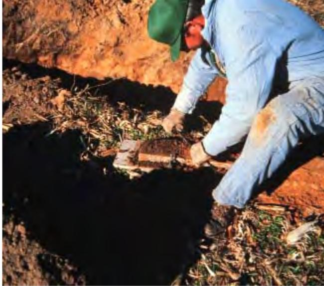
**11.) Carefully cut away, shave, or otherwise remove all soil above the cutting edge of the frame; a machete is an appropriate tool for this job. This is the surface that will be attached to the mounting board. (At this time the monolith may be transported in the frame if desired).**
