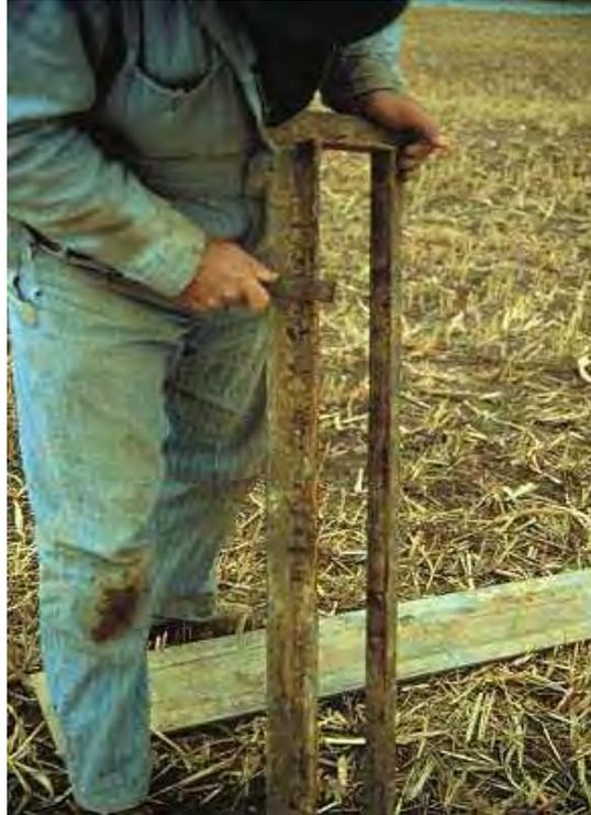
**2.) Place a 2 foot angle-iron frame (with inside dimensions of 4" x 2" x 40") against exposed profile.**
