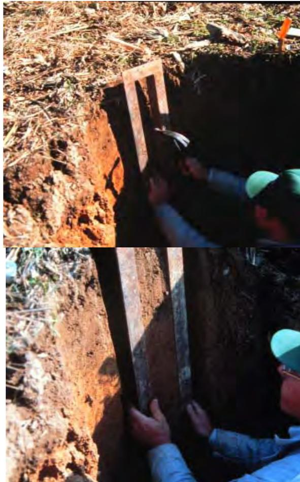
**7.) Depress the frame over the sculptured profile being careful to allow no side- to- side or vertical slippage and maintain constant pressure until profile is free from the pit face.**
