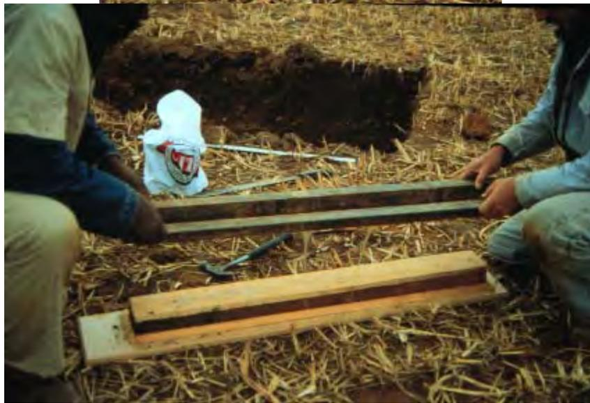
**21.) As the frame is raised about 3/4", quarter-round molding can be placed (tacked lightly) along both sides and ends to hold profile intact until glue has dried. This step may or may not be needed depending on texture, soil moisture content, and disposition of the monolith. Ideally, if molding is used, it should be loosened before glue completely hardens although it can be removed later or allowed to remain.**
