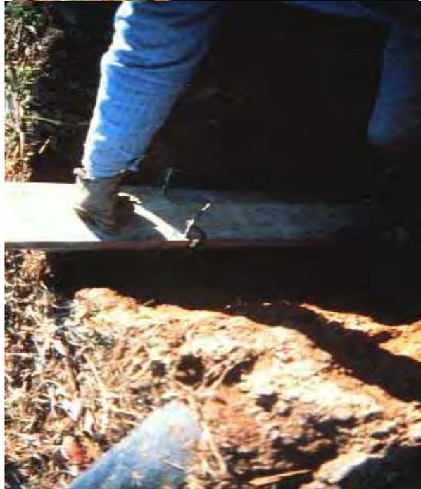
**9.) When both sides are essentially mined to the center, insert a tiling spade at the surface about 4-6 inches beyond the frame and complete the separation of the profile from the pit face. Care must be exercised to insure the sculptured profile does not slip downward or is otherwise pulled from the frame.**
