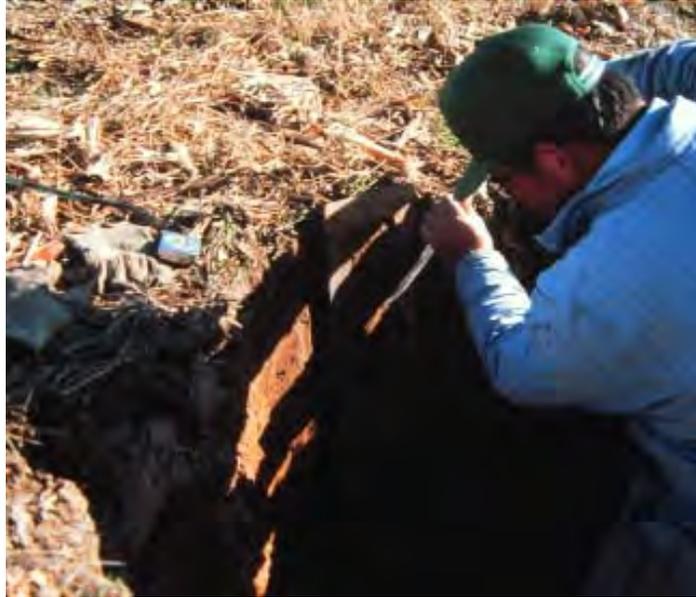
**8.) Excavate along both sides and the bottom of the frame with the objective of capturing 2-6 inches more profile than is eventually required to fill the frame.**
