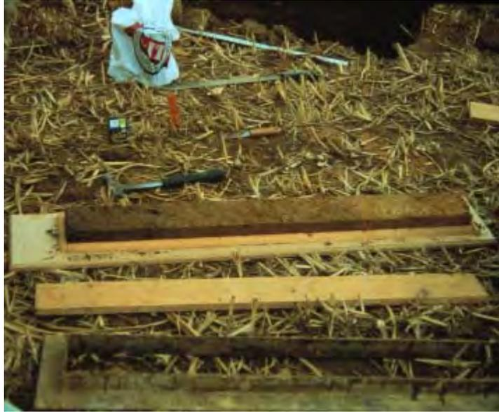
**22.) Ideally, the exposed profile is picked or dressed to show desired structure or finish before the soil dries; however, it can be remoistened for this process. (Dentists' picks, walnut picks, or other fine tools are used for this process . Avoid tool smear marks on finished surface - they will be very obvious on the finished monolith).**
