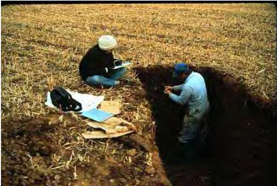
**1.) Excavate pit ( 4 feet deep) - a minimum of about 12 inches additional working space is required on each side of the profile extraction area. Moist soils are nearly essential. Smooth exposed profile face ( this is the face you will eventually pick for your finished profile).**
