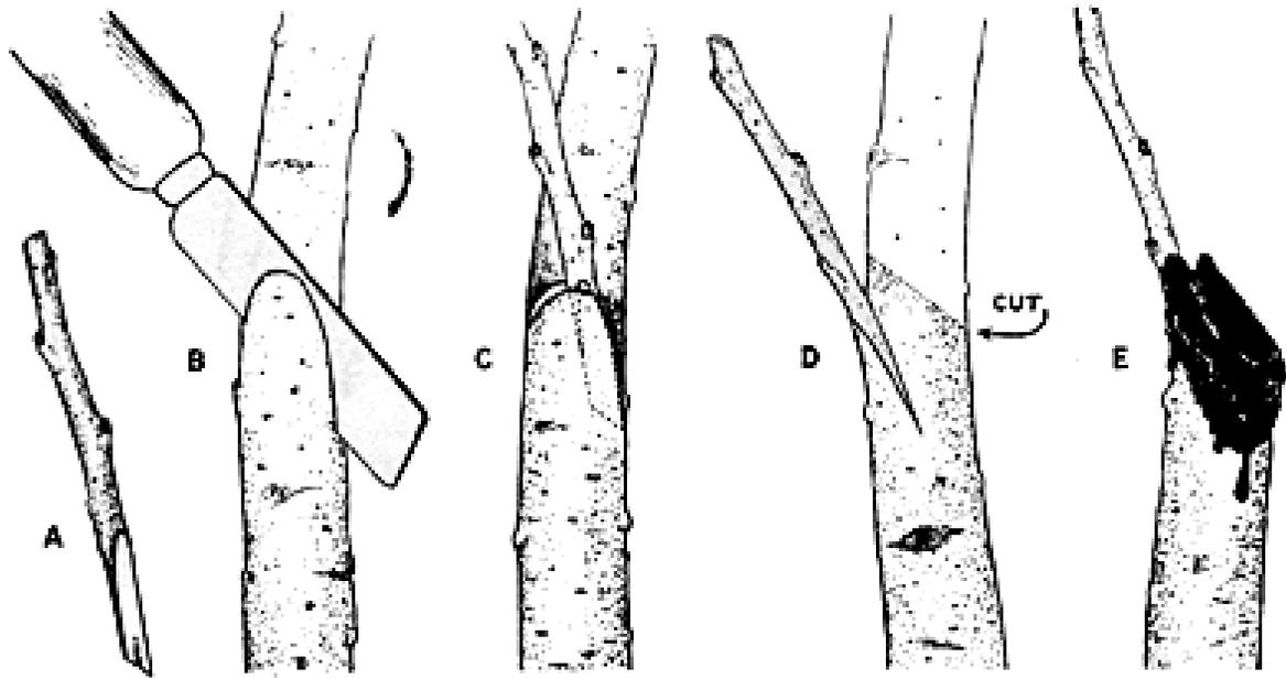
Illustrated here is the side graft. Notice how thin the wedge of the scion is cut. In the second picture a thin bladed saw is used to slice into the branch of a tree. The scion is inserted in the third picture so that the cambium layers matchup. The fourth picture shows a side view and where to cut the second year after the scion has been inserted. In the last picture the branch has been removed and covered with grafting compound.
