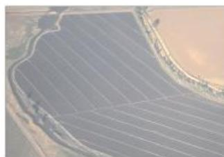
**Figure 2.** Rice field with in-contour levees (left) and straight levees (right) (Source: UCCE Rice Production Workshop 2011).
