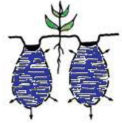
**Figure 2.** Vertical and lateral water movement within soil in furrow irrigation (Source: UC Publication "Furrow Irrigation" by James C. Marr)
