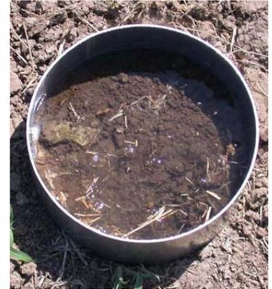
**Figure 1.** Infiltration rate test using a small can or container (Source: USDA).
